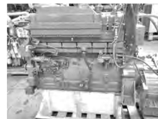
Rebuilt KTA 19 / 3 units
