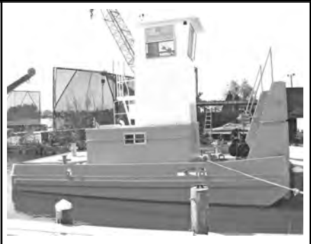
MODEL 2514 25'9" x 14'0" x 4'6" 600 H.P. Twin Engine
