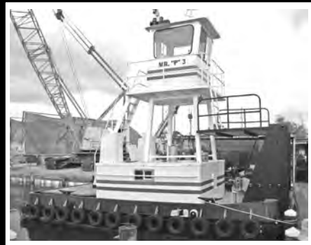
MODEL 2516 25'9" x 16'0" x 5'6" 650-750 H.P. Twin Engine
