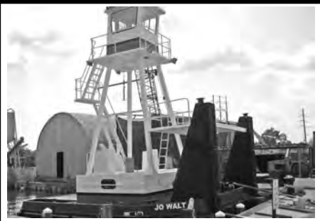
MODEL 2520 25'9" x 20'0" x 6'0" 750 H.P. Twin Engine
