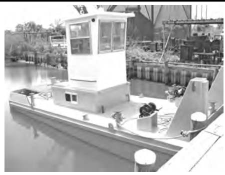
MODEL 2510 25'9" x 10'0" x 4'0" 200 H.P. Single Engine
