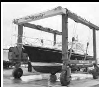
1988 35BFMII - 70,000 lb. Capacity, 17' Inside Clear Width, 18' Inside Clear Height, Ford Gas Engine, Front & Rear Powered Slings. Location - Fall River MA
