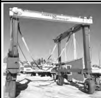
2000 35BFMII - 77,000 lb. Capacity, 17' Inside Clear Width, 18' Inside Clear Height, Ford Gas Engine, Front & Rear Powered Sling. Location - Vinalhaven ME
