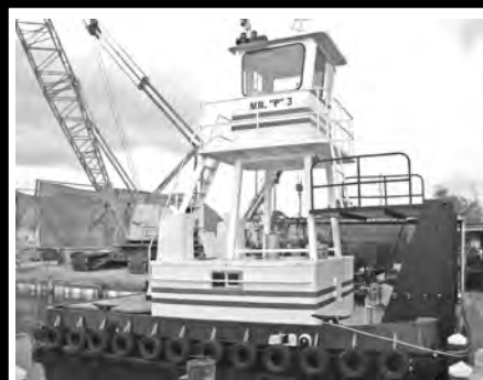
MODEL 2516 25'9" x 16'0" x 5'6" 650-750 H.P. Twin Engine
