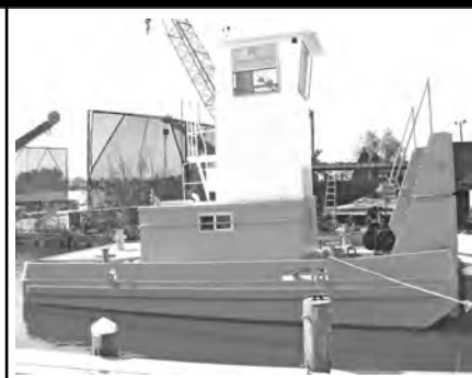
MODEL 2514 25'9" x 14'0" x 4'6" 600 H.P. Twin Engine
