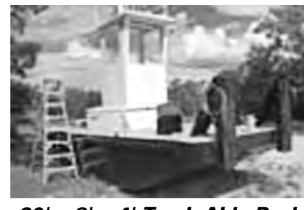
20' x 8' x 4' Truck-Able Push Boat, (1) GM 471, Flanking Rudder, Keel Cooled.
