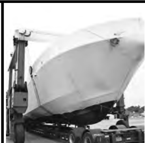
1998 35BFMII - 77,000 lb. Capacity, 18' Inside Clear Width, 18' Inside Clear Height, Ford Gas Engine, Front Powered Sling. Location - Long Island, NY
