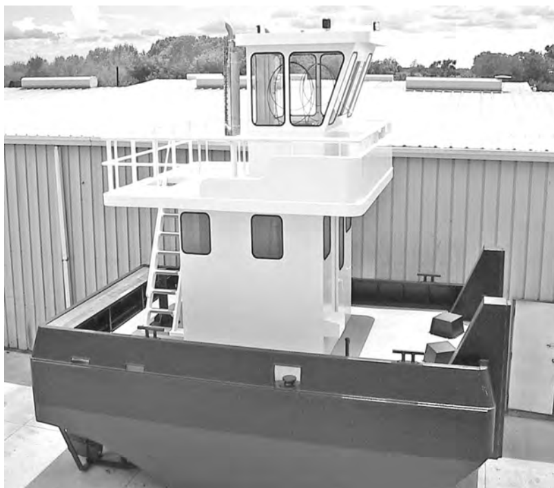
TRIUMPH 25.5' x 14', Twin Screw Towboat, 450 h.p., with Deckhouse, 3.5' Draft.
