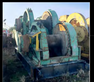
Skagit G160 MAF2581 2,640 ft of 1-1/2 in wire rope 165,000 lbs SLP For Sale | Used
