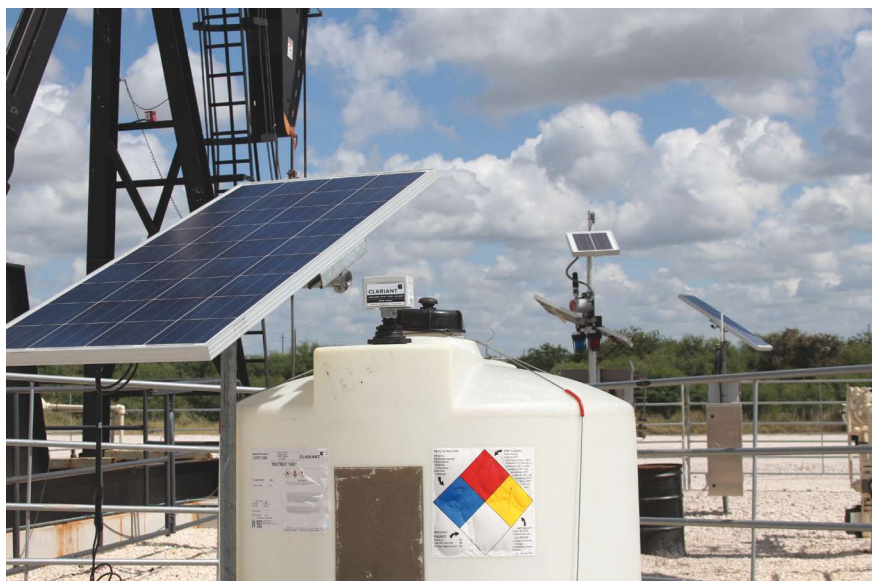
Clariant's remote tank level sensor with a chemical tank is shown. (Source: Clariant)
