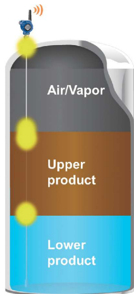
Microwave pulses are sent out by a transmitter installed at the top of the tank. As the pulses travel through the oil (in brown) or water (in blue), the actual level measurement is taken as a function of the time taken from when the signal was emitted to the time at which the echo from the media (be it oil or water) is received. (Source: Emerson Automation Solutions)
