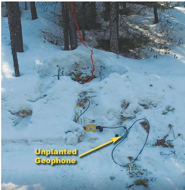
A drone-conveyed camera recorded this receiver station where the geophone is not properly planted. (Source: Geospace Technologies)
