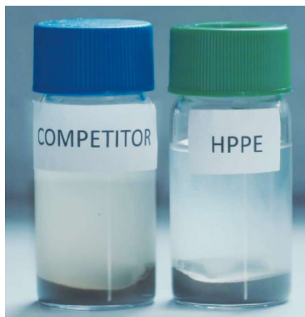
FIGURE 1. In this clay pack test filtrate comparison there is a significant amount of migrated fines with a leading clay control product. With the HPPE CS series, the effluent is clear. (Source: HPPE LLC)
