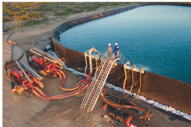
Water sourced from an underground aquifer is transferred via aboveground pipeline to a MAG Tank in West Texas. (Source: Fountain Quail Energy Services)
