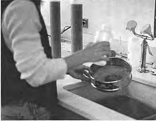
Figure 24. Wet sieving silt and clay particles from one of the samples from site 34RM507.
