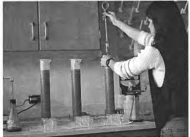
Figure 25. Doing a pipette draw on a sediment sample from site 34RM507.
