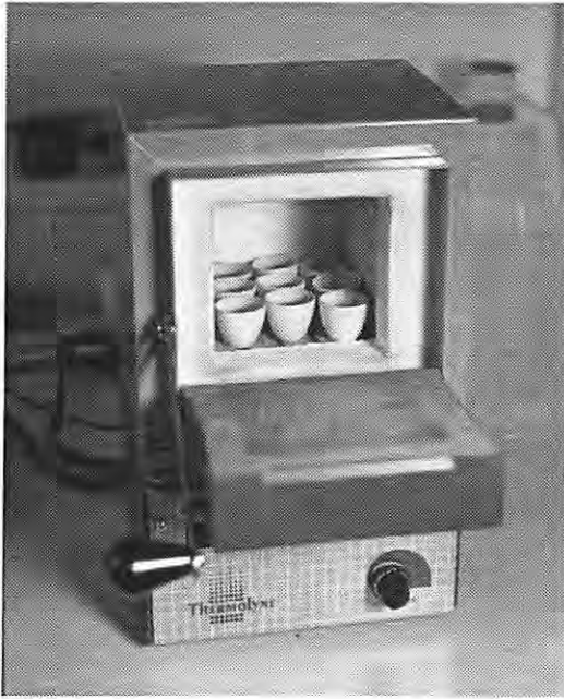
Figure 22. Burning sediment samples in the muffle furnace to gather data on weight loss on ignition..
