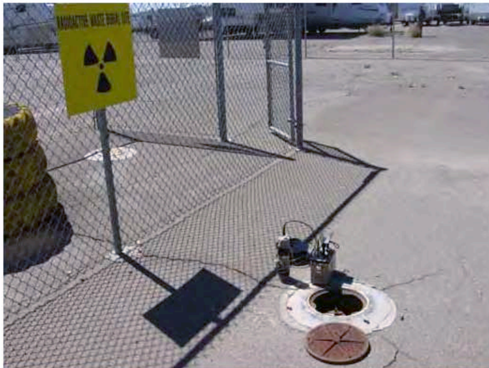
Photograph 2: The Ludlum Model 2221 portable scaler/ratemeter and Model 44-10 scintillator probe next to monitoring point MP-4.
