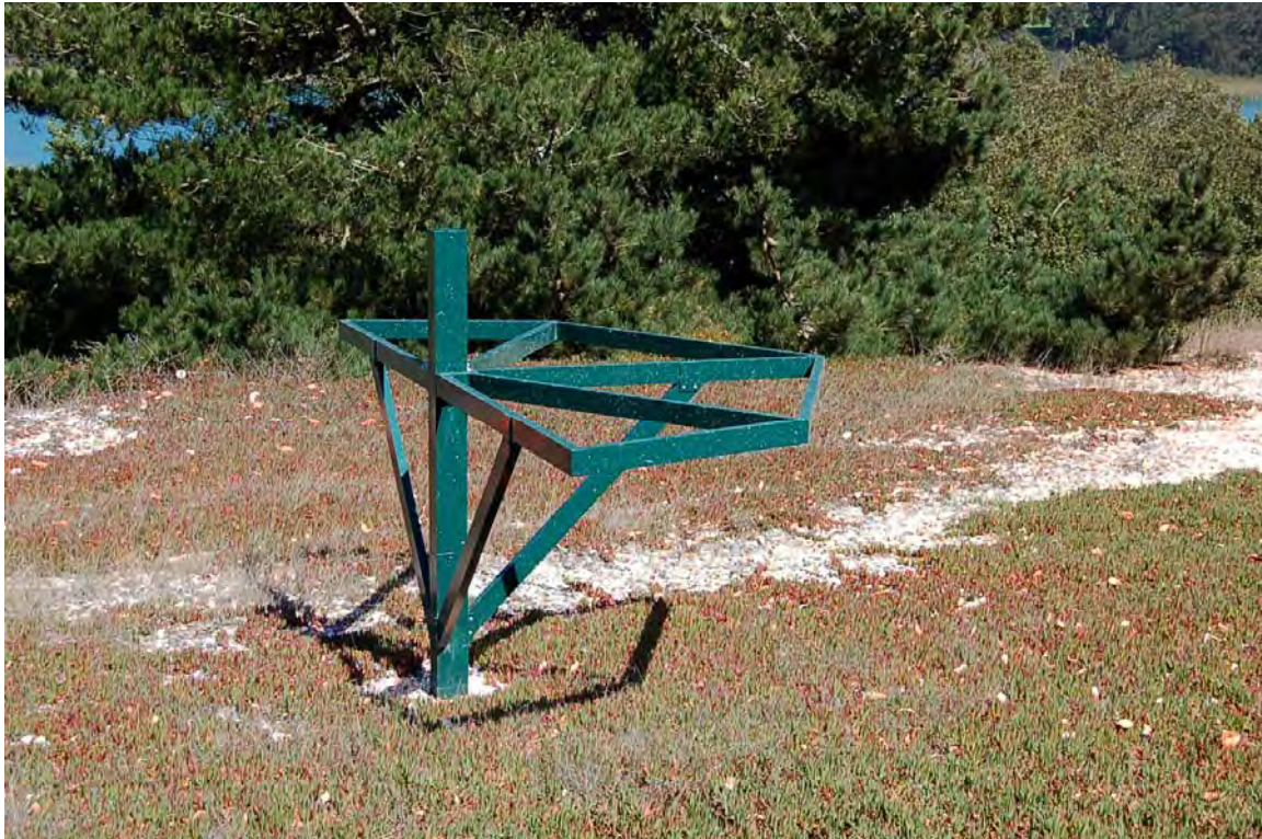
Photo 20. One of two landing posts (used to calibrate Olymic Skeet machinery for Field 7) located in the outfield area NE of Field 7 (D. Bradley, September 2013).
