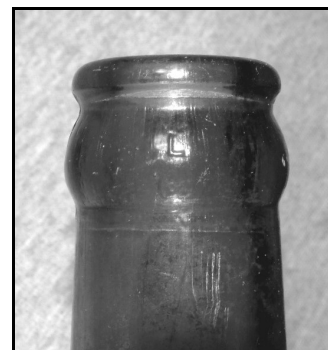
Figure 10b-23 – Tiny “L” on the reinforcing ring of the crown finish
