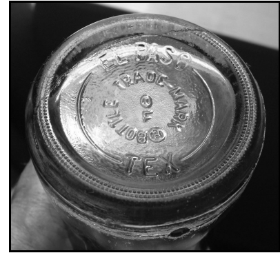
Figure 8-96 – Original Random Baseplate format – central embossing refers to the bottle trademark
