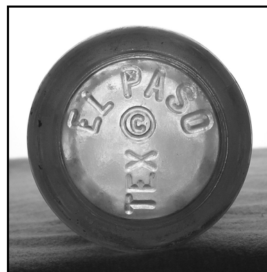
Figure 8-99 – IN U.S. PATENT OFFICE transitional base – Chattanooga Glass Co.
