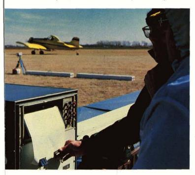
of nozzles. In the latter case, the applicator can make on-the-spot adjustments (right) and recheck his pattern. Other users of the OSU system include agricultural aircraft manufacturers seeking to develop or improve dispersal systems for their aircraft.
