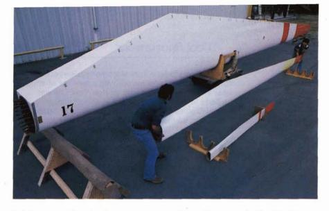
The large blade in the picture is a 60-footer developed for NASA; the smaller blades are Gougeon products manufactured for commercial wind turbines that provide electricity for homes, farms, apartment complexes and small utilities.
