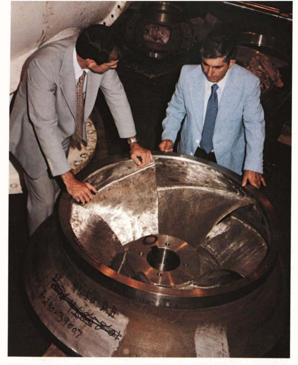
COSMIC-supplied computer program known as MERIDL. The program makes flow analysis calculations that permit designers to evaluate the performance and efficiency characteristics that can be expected from the pump's impeller. MERIDL also provides information that enables a trained hydraulic engineer to make design improvements.
