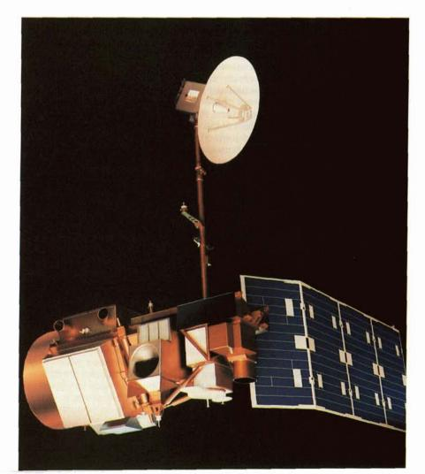
On the opposite page, the Landsat-D satellite is undergoing tests in a clean room facility at General Electric Company's Space Systems Division. Weighing more than two tons, it is an advanced member of the Landsat family of Earth resources monitoring satellites in service for a decade. At left, Landsat-D is pictured as it will look in orbit, with its antenna and solar cell array extended.
