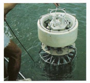
The monitor demonstrated its ability to provide voluminous water quality data in a seven-day field test at Saginaw Bay, an eastern Michigan arm of Lake Huron, In these tests, the system used only one-third of its battery energy supply, indicating that it could function well beyond the design goal of two weeks. On completion of the field tests, the monitor was turned over to EPA's Large Lakes Research Station, Grosse Ile, Michigan.
