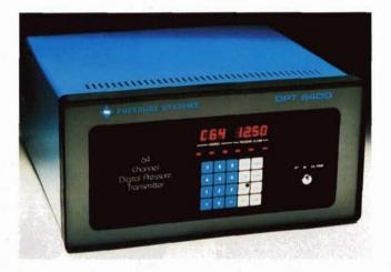
plant's process control computer. The DPT 6400 serves that function; by employing solid-state pressure-sensing transducers whose errors are automatically corrected by a microprocessor, it is capable of highly accurate pressure measurements; above, the digital reading (in red) indicates the channel number and the pressure, in pounds per square inch, at the loop being sensed. The basic DPT 6400 has 64 channels, but the system can be expanded to 256 channels by addition of "slave" units.
