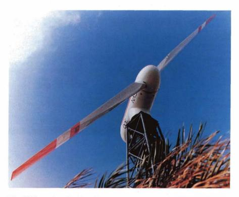
This NASA-developed wind turbine generator in Hawaii provides enough electricity for 100 homes. Its wood composite blades were made by Gougeon Brothers Inc., a Michigan sailboat builder which has also become a leading firm in commercial wind turbine manufacture.
