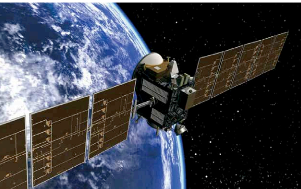
NASA's Dawn spacecraft used a high-efficiency ion thruster to visit Ceres and Vesta in the asteroid belt. This electric method of propulsion is now being manufactured for small satellites by Orbion Space Technology. Credit: NASA
