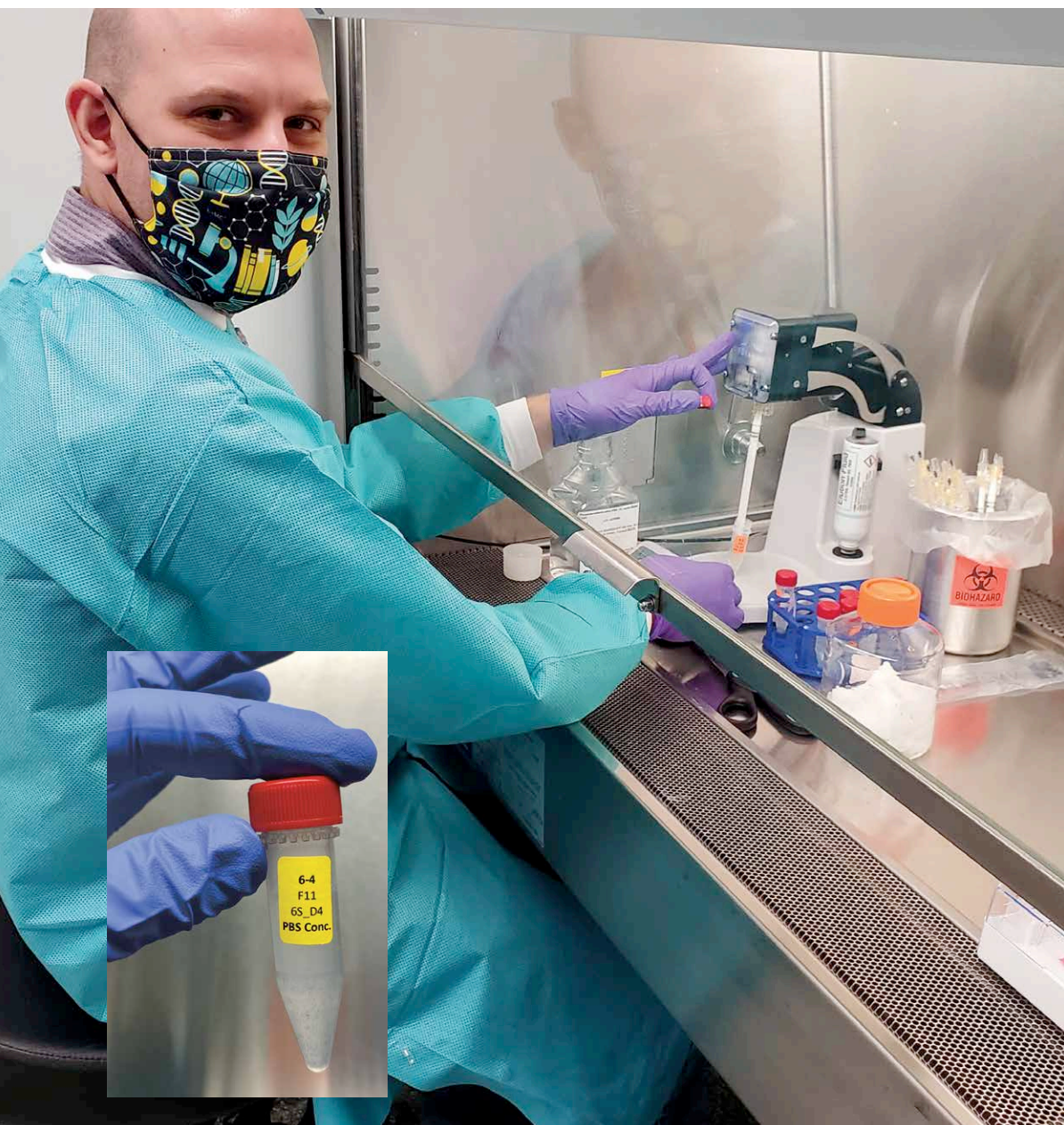
After the cloths used to wipe down the space station arrived on Earth, they were rinsed in the water jar seen here with an orange lid to remove microbes. That liquid was then concentrated into this vial (inset) for testing by InnovaPrep's CP Select system. Credit: NASA
