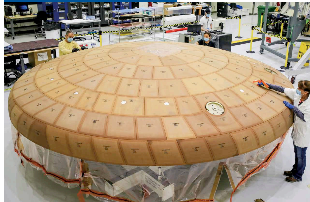
Technicians at Kennedy Space Center finish applying blocks of Avcoat, a lightweight epoxy resin, to the heat shield for the Orion crew module. To examine the blocks' bond to the shield, NASA turned to Aerospace Corporation to develop an ultrasonic sensor that could spot defects in or under the material despite its resistance to sound. Credit: NASA
