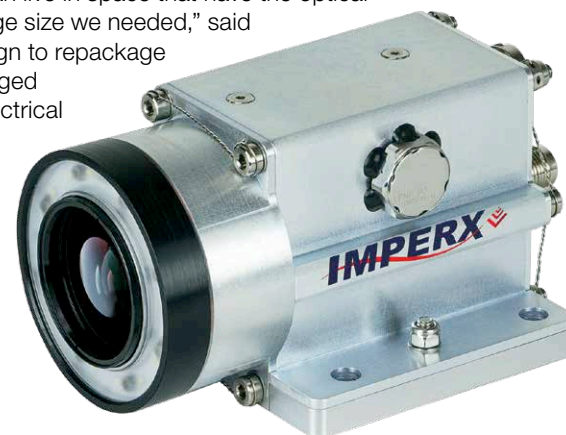
Specifically designed for launch vehicle applications, the Imperx SPC-S2010 camera employs NASA-developed ruggedized housing and internal electronics design. The camera has an internal heater and an integrated LED illumination ring that supports continuous lighting. Credit: Imperx Inc.
