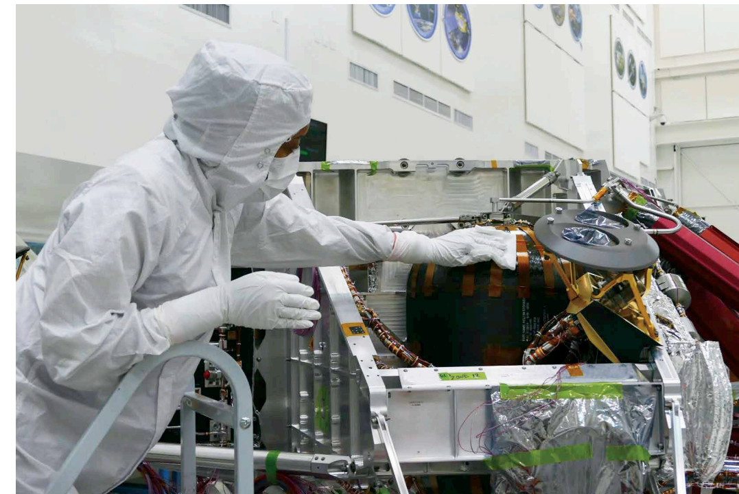
Wiping down the hardware of the Perseverance rover is one step in NASA's Planetary Protection strategy to limit the number of Earth microbes going to Mars. The Jet Propulsion Laboratory cleanroom, one of the cleanest places on the planet, developed procedures using InnovaPrep technology to check for any microbes left on the surface before flight. Credit: NASA
