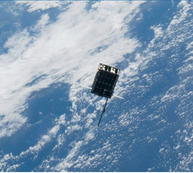
The Dellinger CubeSat falls into orbit shortly after its release from the International Space Station in 2017. The antennas on the small satellite were deployed as a test of the Diminutive Assembly for Nanosatellite Deployables (DANY) mechanism, which was later developed into the Gecko Actuator. Credit: NASA
