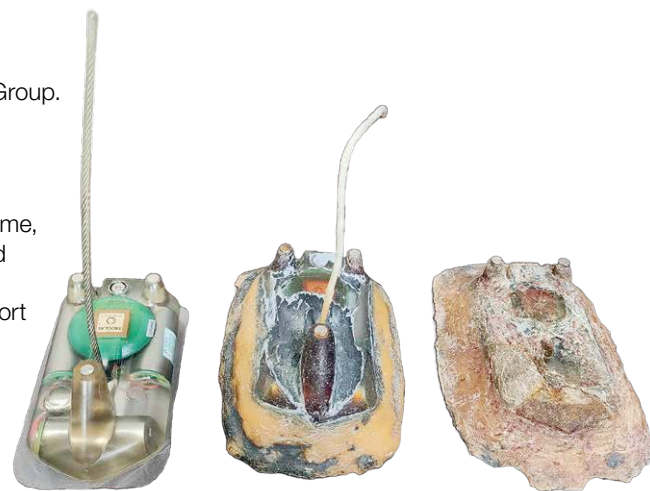
Transponders designed to attach to the shell of a sea turtle are lightweight, so they don't interfere with the animal's ability to swim. The base (left) records and retains sensor data, transmitting the information along with a GPS signal when a turtle surfaces. As the shell sheds layers, the transponder falls off, like this one found in the Florida Keys (right) or can be safely removed from a nesting turtle (center). Any stored data can then be downloaded. Credit: NASA
