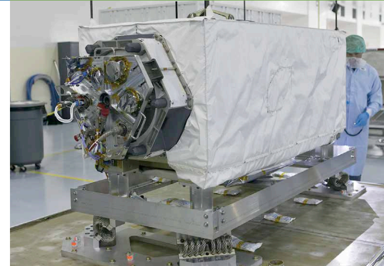
One of IrriWatch's sources of data is the Ecosystem Spaceborne Thermal Radiometer Experiment (ECOSTRESS), seen here undergoing inspection at Kennedy Space Center prior to launch. Built at the Jet Propulsion Laboratory and affixed to the outside of the International Space Station since 2018, ECOSTRESS is the first Earth-imager developed specifically to look at evapotranspiration, a major indicator of plant stress. Credit: NASA
