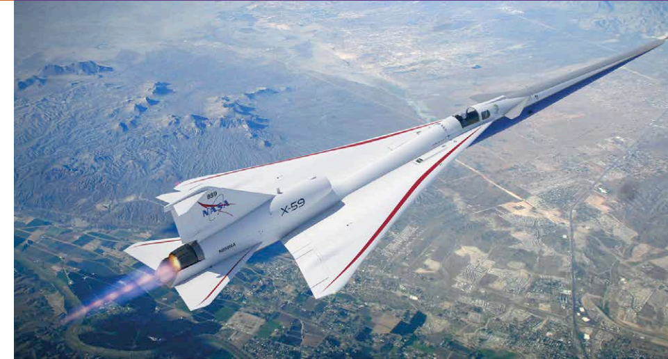
When a plane reaches the speed of sound, it creates a sonic boom so loud that commercial supersonic flight is banned over land. NASA redesigned the traditional airplane shape to reduce the boom to a "thump," relying on video cameras to replace the front windshield. Credit: Lockheed Martin Corp.
