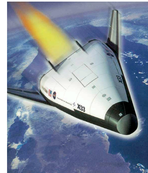
The Lockheed Martin X-33 X-plane, shown in this artist's rendering, was intended to demonstrate technology pioneered under NASA's Reusable Launch Vehicle program in the 1990s. The program was cancelled in 2001, but an emissive heat shield coating invented at Ames Research Center under the initiative has since found widespread commercial success as the Emisshield product line. Credit: NASA
