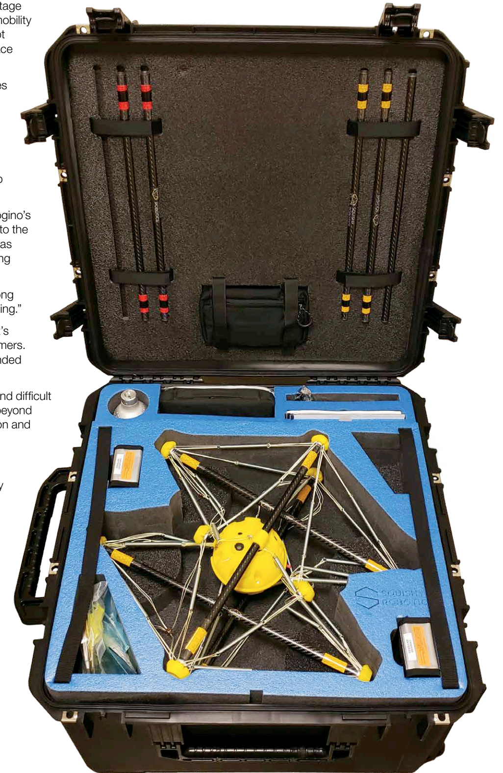
Tensegrity robots can be “squished” down for easy packing and shipping – a feature that’s especially interesting to NASA because there’s not much extra room on spacecraft. Credit: Squishy Robotics Inc.
