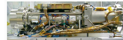
The Tunable Laser Spectrometer on NASA's Curiosity Mars rover bounces a laser 81 times through a chamber filled with sample gas. This measures absorption of varying laser wavelengths to determine not only concentrations of different gases but also their isotope ratios, which give clues about the sample's history. Funding and expertise from NASA have helped a company develop a much smaller commercial version of the technology. Credit: NASA
