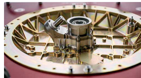
Orbion's Aurora thrusters are small and efficient yet powerful enough to maintain the orbits of small satellites for several years. Credit: Orbion Space Technology Inc.
