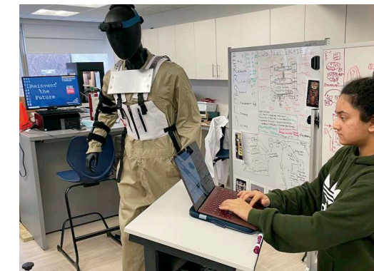
Agha performs testing on NASA's upper body robotic exoskeleton, a soft, wearable robotic garment designed to control the shoulder and elbow. It was originally developed to provide motor rehabilitation for patients with neurological impairments, such as brain injury or stroke. Credit: NASA
