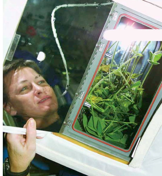
Astronaut Peggy Whitson checks on soybean plants growing in the Advanced Astroculture plant-growth chamber, which went into use on the International Space Station in 2001. The NASA-funded Wisconsin Center of Space Automation and Robotics invented an ethylene scrubber that kept the plants from withering prematurely and became the basis for Fresh-Aire UV's air purifiers. Credit: NASA
