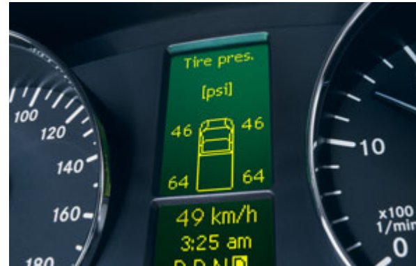
Tire pressure monitoring system (standard for Cargo Van and Passenger Wagon; not available in conjunction with Chassis Cab or twin tires)
