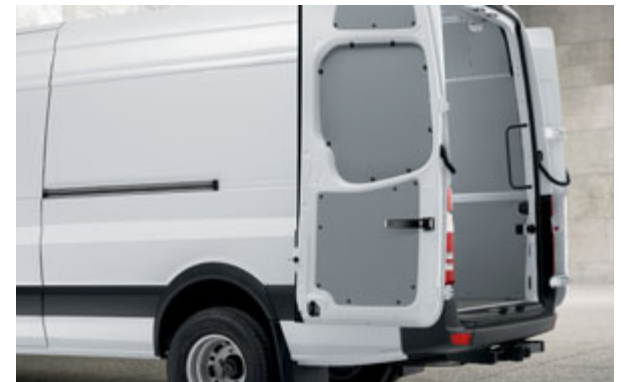
Hinged rear doors which open up to the side wall (and lock into position automatically) are available as standard equipment
