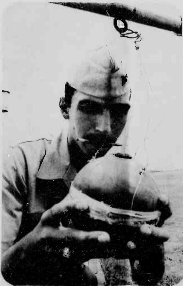
Corporal Bob Bennett reads temperature on a globe thermometer. This particular thermometer helps determine temperature ranges suitable to the human body. When the temperature reaches certain levels, the weather service issues warnings to units to cease or cut down on physical activities that may be hazardous if continued under high temperature conditions.
