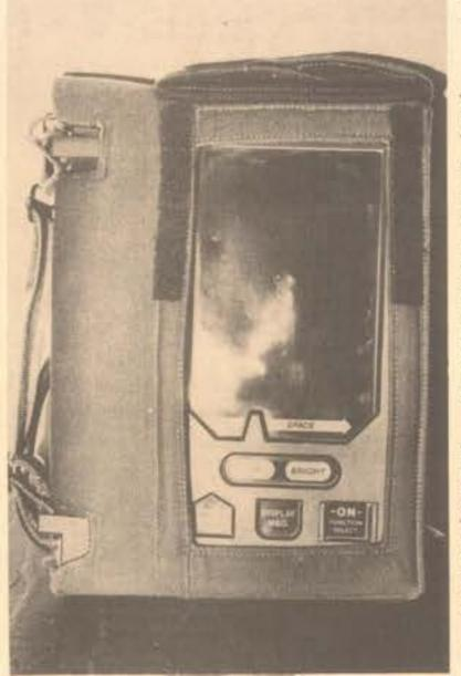
NEW WAYS TO MAKE WAVES -The Digital Communications Terminal will revolutionize field communications for the Marine Corps through the use of burst transmission. The DCT scheduled to reach infantry units by 1985, will enable Marines to communicate easier. and faster than ever before.
