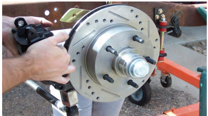
Mike installs calipers on front in brake class.
