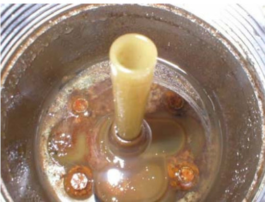
Corrosive fungus, algae and bacterial growth in secondary fuel filter housing and high pressure pump volume control valve.
