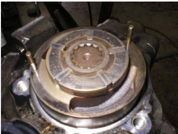
Excessive water in the fuel led to this corrosion in the High Pressure Fuel Pump Internal Transfer Pump and on the Fuel Volume Control Valve
