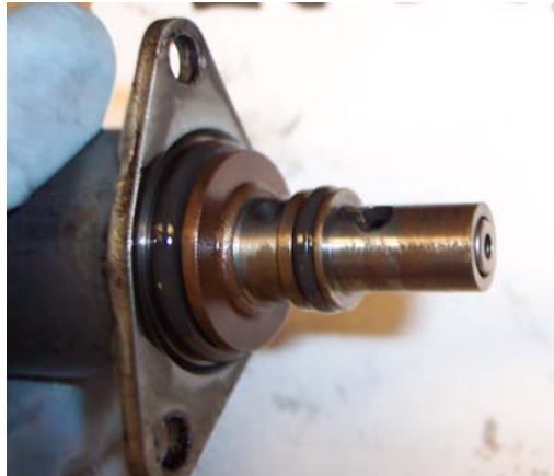
Excessive water in the fuel led to this corrosion in the High Pressure Fuel Pump Internal Transfer Pump and on the Fuel Volume Control Valve
