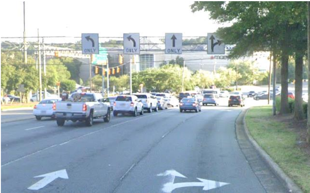
Figure 18. Arterial OLCS, Southbound SH 50 at US 70, Raleigh, North Carolina.
