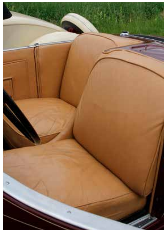
Of the five different body styles offered for the 734 series of 1930, only the two-passenger runabout (boattail) featured the staggered seating. "The driver's seat being placed slightly forward of the passenger's seat, s in a racing car to insure the driver against any interference when traveling at high speed." — PACKARD NEWS SERVICE
