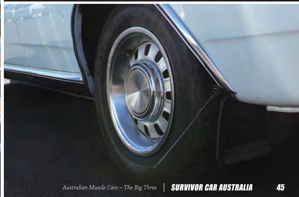
Above left: The introduction of the scoop was a pretty daring and bold design by 1960 standards. Left: It's hard to find an early Falcon that has never experienced battery splatter on the engine bay paintwork. Bottom left: The original log books are kept safely in the glovebox. Below: Do you know what this does? It scrapes the curb when parking so you know your distance is spot on.
