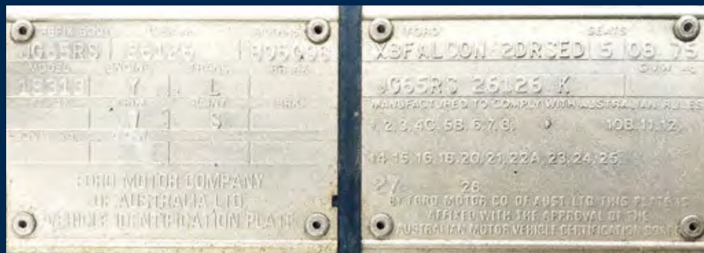
Above: If you've found a 1975 XB Falcon hardtop with a model code 18313, and a chassis number prefixed with JG65R, which has the engine code 'Y' on the identification plates, with either an 'L' or 'B' code for the transmission, and either an 'S' or 'Q' as the paint code, then you're heading in the right direction towards verifying it as a John Goss Special.
