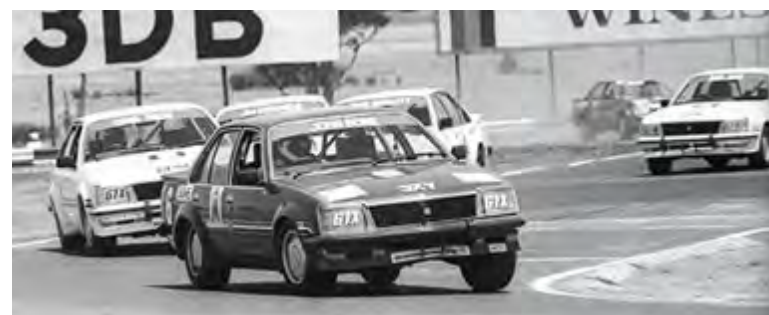
Wheel arch flares, three piece rear spoiler, and Irmischer wheels, all of a sudden the humble Commodore starts to resemble a race car!
