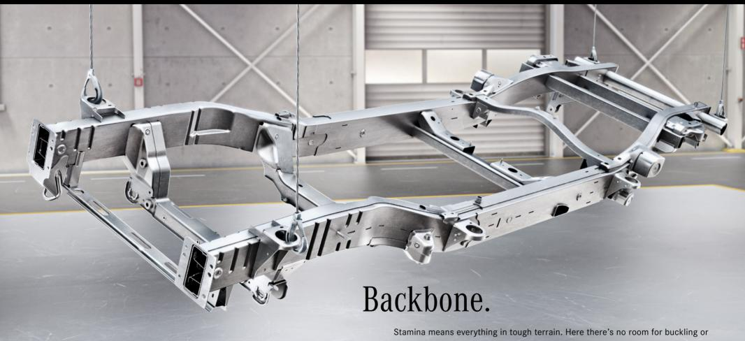
retreating. Here it's all about character. And strength of character shines through in the vehicle's backbone. In the case of the G-Class, this has always been the exceptionally robust ladder frame. Made from sheet steel up to 3.4 mm thick, the ladder frame is much more suitable for tough off-road use than a self-supporting body. In addition to this, the decoupling of the noise from the suspension and the road reduces the interior noise level and thus enhances the ride comfort.
