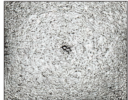
Spontaneous breakage in thermally tempered glass due to nickel sulfide inclusion
