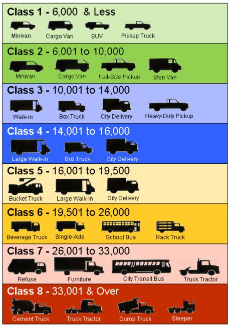
FIGURE 75. Examples of Trucks in Each Truck Class
