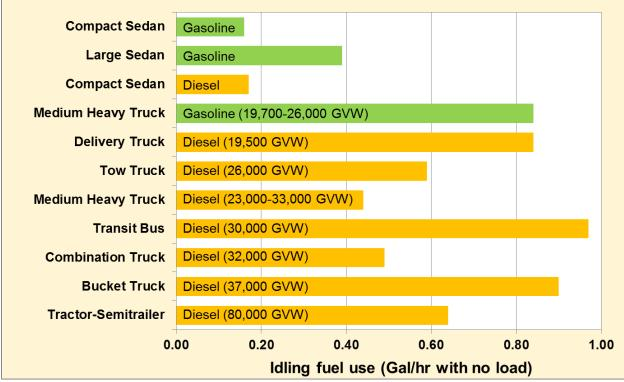
FIGURE 87. Fuel Consumption at Idle for Selected Gasoline and Diesel Vehicles
