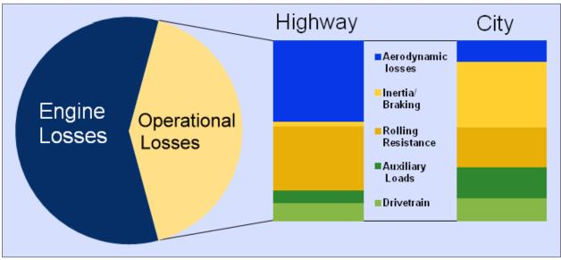
FIGURE 110. Class 8 Truck-Tractor Energy Losses
