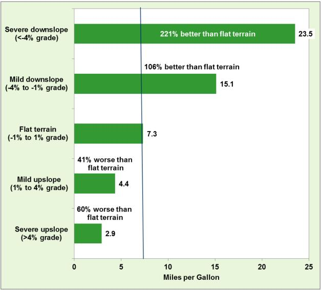
FIGURE 86. Fuel Efficiency of Class 8 Trucks by Roadway Grade
