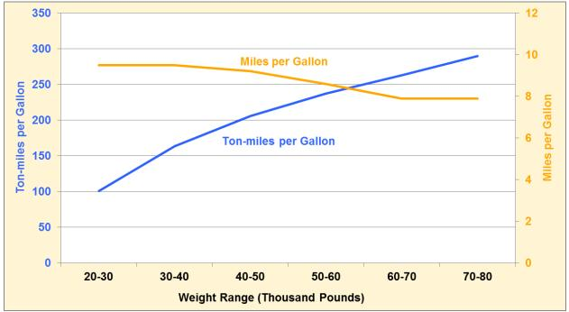
FIGURE 85. Fuel Efficiency of Class 8 Trucks by Vehicle Weight Range on Flat Terrain at 65 mph
