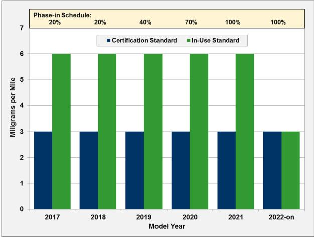
FIGURE 125. Tier 3 Particulate Matter Emission Standards for Light Gasoline Vehicles, MY 2017 and Beyond
