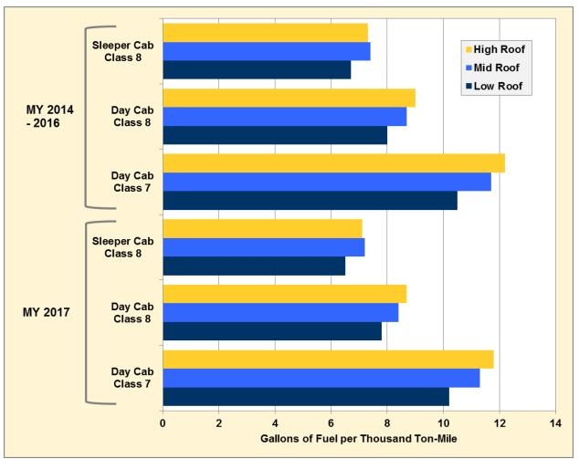
FIGURE 127. Fuel Consumption Standards for Combination Tractors, MY 2014-2017
