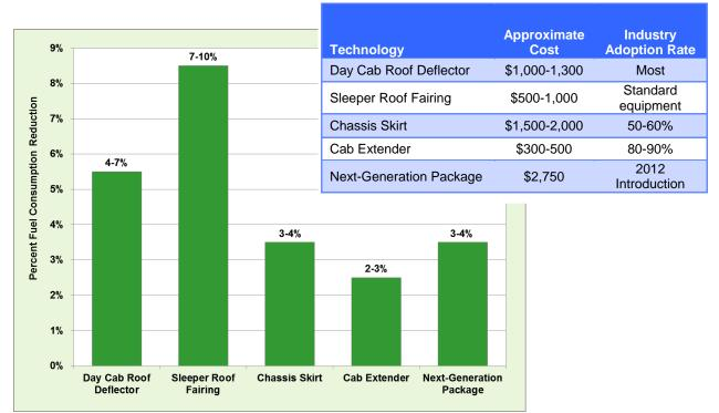
FIGURE 111. Fuel Consumption Reduction Rate, Approximate Cost, and Industry Adoption Rate for Aerodynamic Technologies
