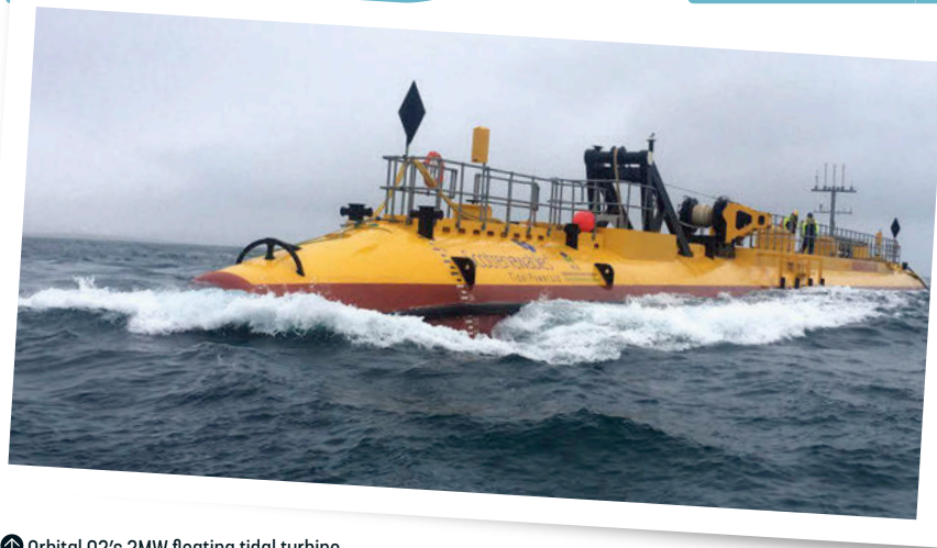
Orbital O2's 2MW floating tidal turbine
