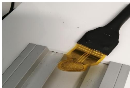
Figure 14. Kapton sensor with a double spiral conducting.
