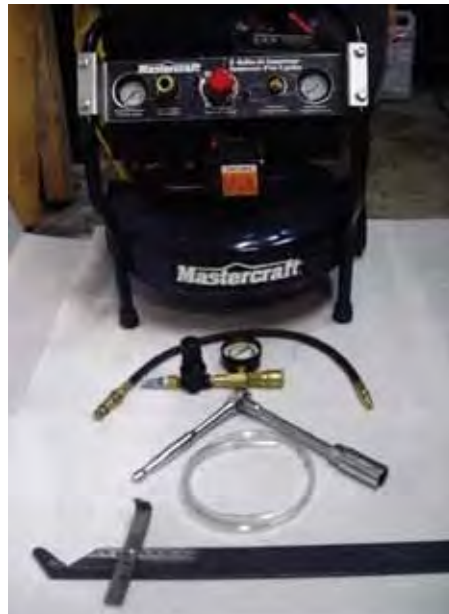
The Leak Down Test gear includes a compressor, a quick connect/disconnect hose attachment with brass spark plug adaptor, air regulator and other minor bits and pieces.
