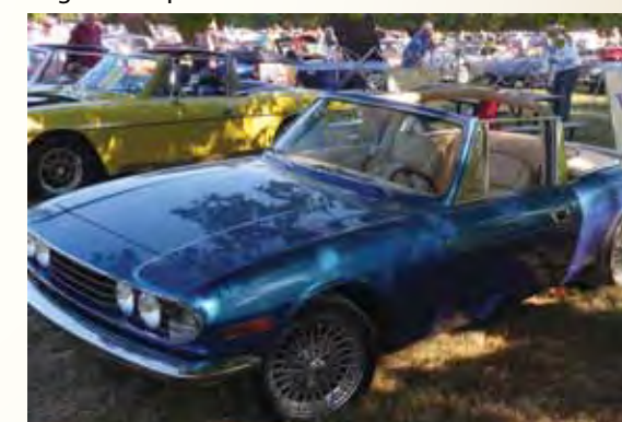
Mk 1 Stag, this particular car has the Rover V-8 engine, 16 inch wheels and colour-matched trim on the T-bar brace. The brace was considered an advantage in meeting potential U.S. safety regulations for convertible cars
