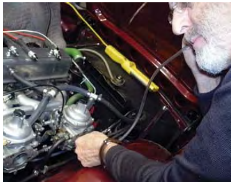
Intake valves can be checked by lifting the carburetor piston and inserting the tube into the intake side of the carburetor.
