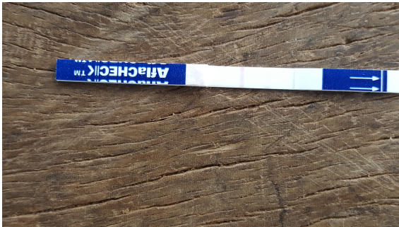
Fig. 8. Test strip showing a single red line implying a positive test ( > \text{or} = 10\text{ppb} ).
