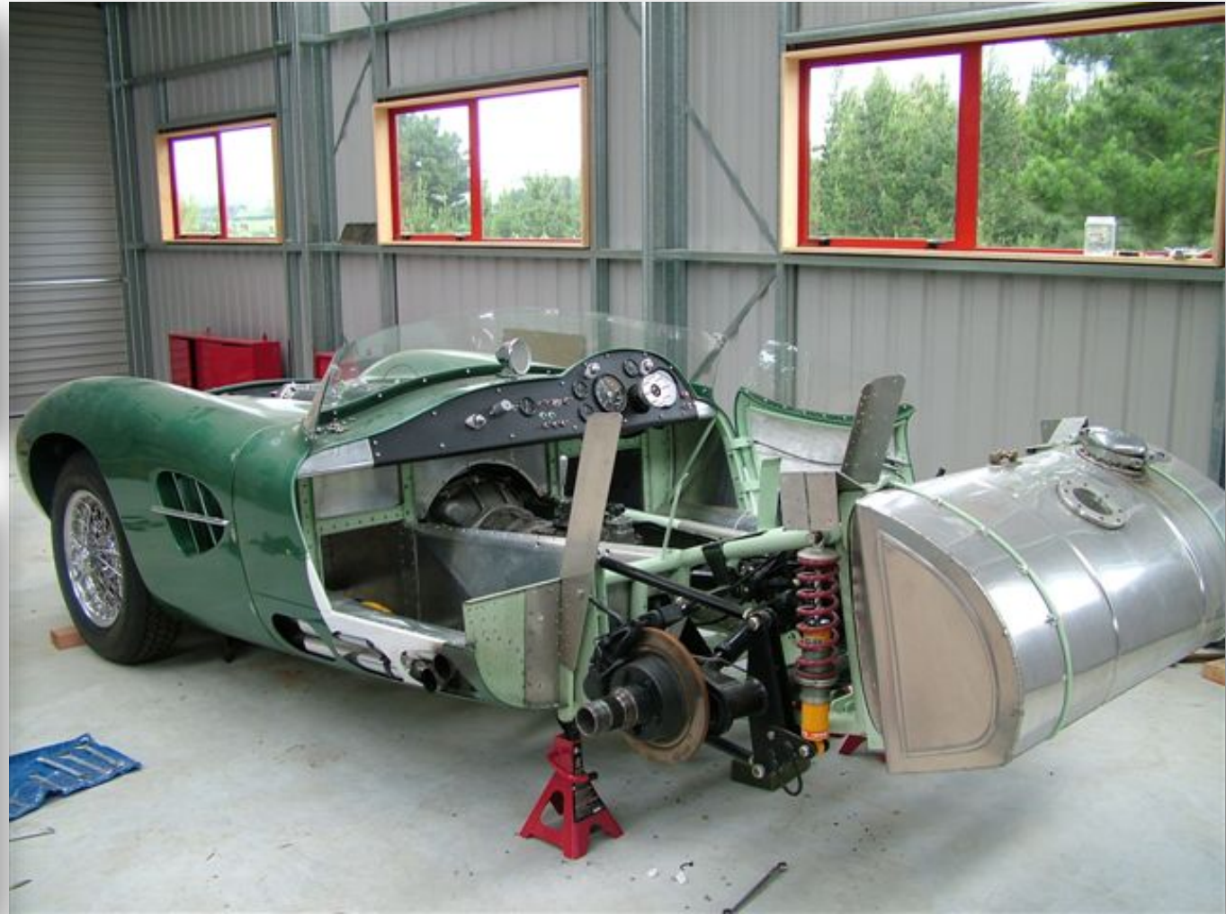
Rear end showing De Dion Rear End and 165 litre Fuel Tank
