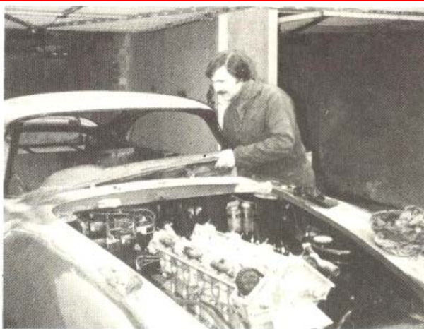
Tim struggles to fit the dash during his rebuild of the 'river car'. Note the new roof that had to be made. The engine was rebuilt to racing spec, but incorporating Tim's ideas so that the Aston could still be driven on the road.
