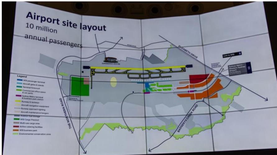
The initial layout allows for 1 runway and 10 million passenger movements a year. The site will be expanded to 2 runways and additional terminal space over the following decades to allow around 80 million passenger movements a year
