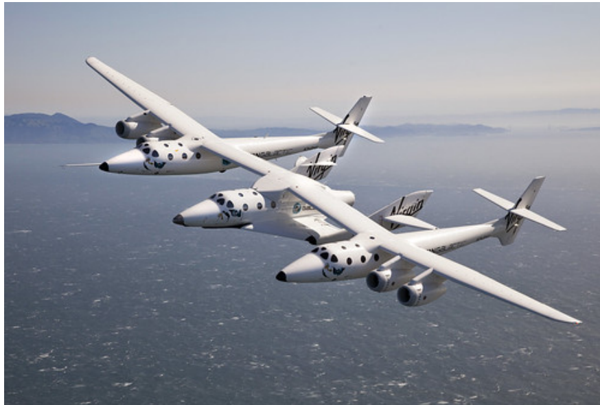
Figure 3.6: VSS Unity attached to its twin-boom carrier mothership, the VMS Eve
