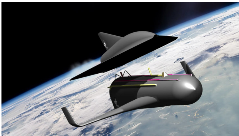
Figure 2.8: SpaceLiner conceptual aircraft composed by two stages
