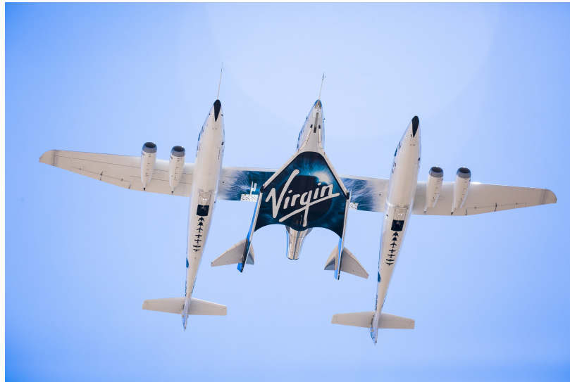
Figure 3.2: SpaceShipTwo spacecraft and its carrier aircraft WhiteKnightTwo
