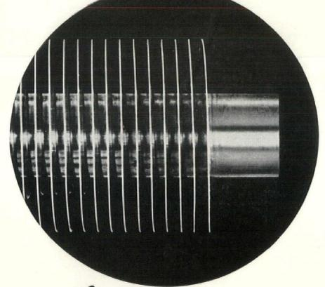
Aerofin smooth fins can be spaced as closely as 14 per inch with low air friction. Consequently, the heat-exchange capacity per square foot of face area is extremely high and the use of high air velocities highly practical. Tapered fin construction provides ample tube-contact surface so that the entire fin becomes effective transfer surface. Standardized encased units are arranged for simple, quick, economical installation.
