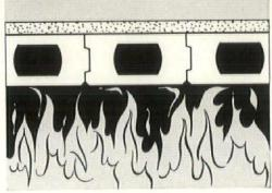
In fire tests conducted by Underwriters' Laboratories, Inc., the Doxplank tested received a 4-hour rating as a noncombustible material.
