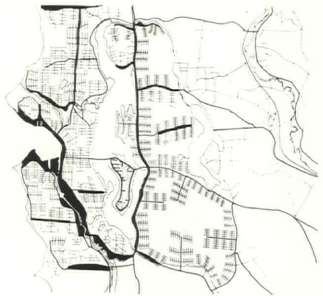
Intermediate Stage. The stage of transition. To the existing local highways new traffic arteries are added. This highway network will eventually form the boundaries of the future communities, into which the city will be subdivided. These traffic arteries will attract commercial and industrial establishments and the areas along the arteries will be zoned accordingly. Within the residential area some streets will be removed, others closed, in order to prevent through traffic.
