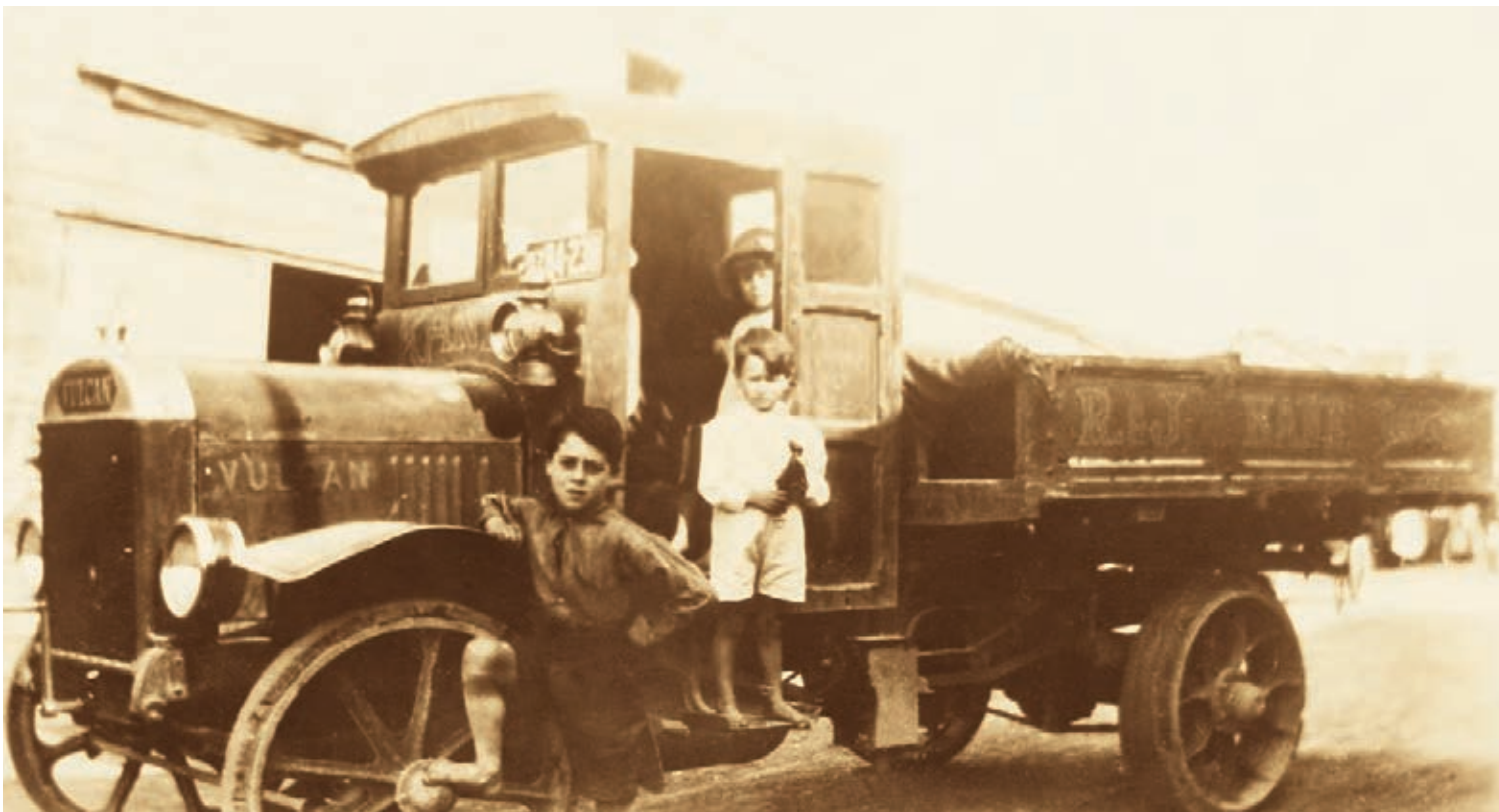
Photo taken in 1925 or 1926 showing the Kane children, Mercia in the cab, Jack on the step and Eric. This Vulcan has the split screen and door at back of cab. The Mascot has not been stolen, electric headlights fitted and you can see the hoist pump by Jack's leg.
