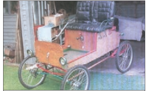
REPLICA OF ONE OF BAKERS FIRST BATTERY CARS. Two seater of about 1900. It has tiller steering and chain drive and can travel up to about 10 miles at about 10mph on 12 volt battery. Calling for offers. Phone Roy 09 267 6644. MEM
