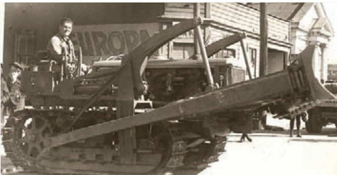
Early dozer with hydraulically operated blade outside Premier Garage in Greymouth, Lofty Johnson at controls.
