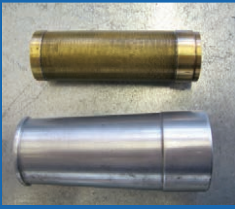
Above: All-metal full-flow filter from a Bugatti.
