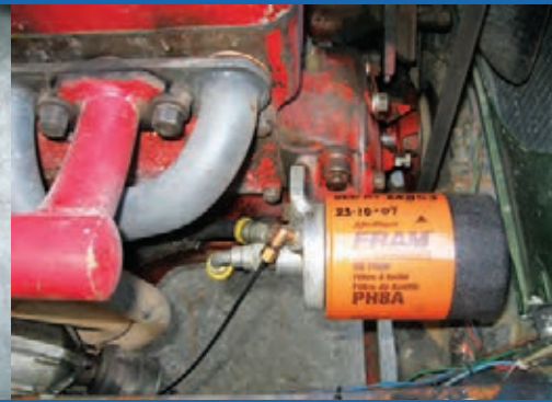
Full-flow filter with a pressure conversion on a model A Ford
