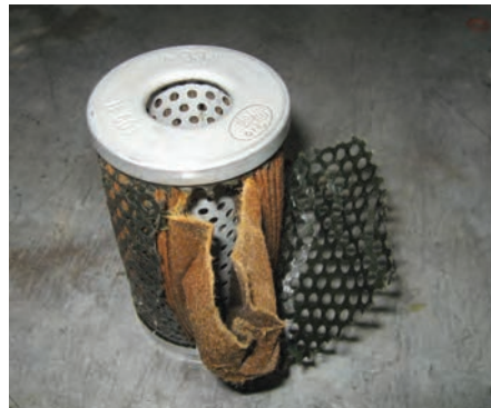
What happens when you try to pass oil through a filter in the wrong direction.
