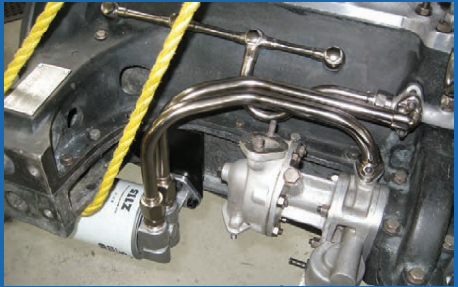
Right: Full-flow filter conversion on an Alfa Romeo P3.
