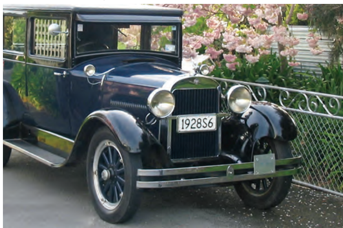
1928 Essex Coach – A feature of the Essex is its all steel body and a single very long door hinge. Many of these models were in common use as taxis in the late '20s and early 30s. This example is owned by Alistair and Mary Howard, Feilding.
