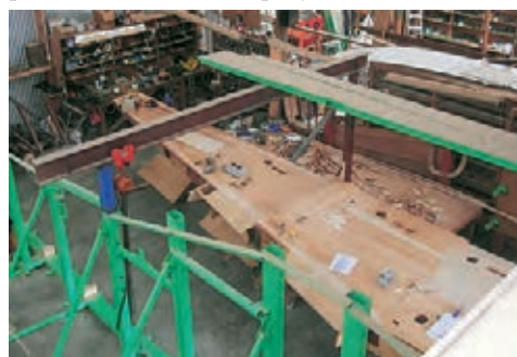
Northland: Mosquito wing under construction at Glyn Powell's
