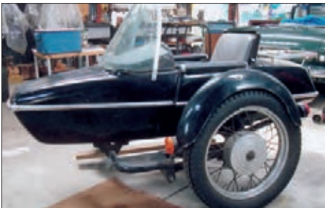
SIDE CAR tube chassis, cable brake. Trailing arm suspension, 18 inch wheel. Steel body mounted on rubber blocks. Top of nose section slides forward for entry. $950. Phone Brian 09 236 0691 MEM
