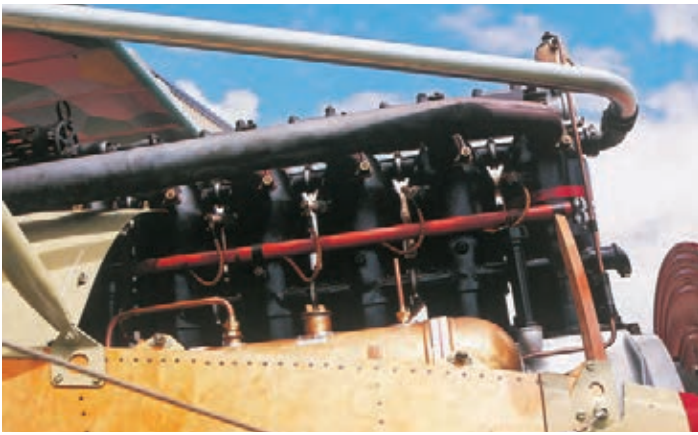
Mercedes Definition: Six separate cylinders and the single overhead cam practically defined the WWI German in-line engine. The upper pipe is to the wing-mounted radiator.
