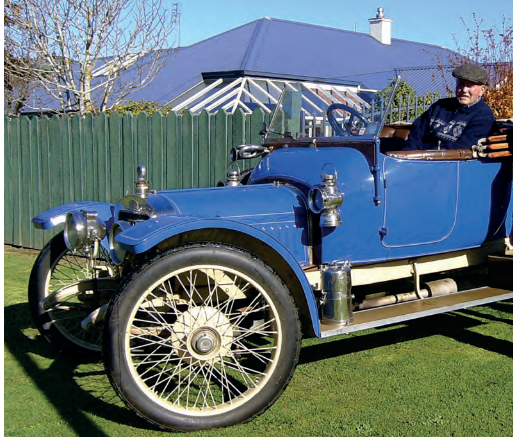
Colin and Joan Pearce in their 1912 Sunbeam 3 litre. The motor has a non-detachable cylinderhead which made removal of pistons and conrods in the seized motor very difficult.
