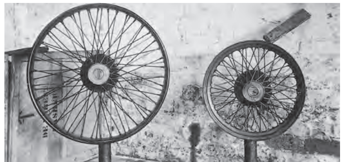
Left original Daimler wheel. Right a new wheel built on the Daimler RW 80 splined hub. Both same distance from camera.
