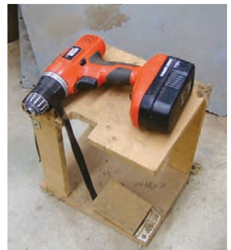
Howard's device for using the power drill. A foot-pedal operated band holds the chuck still while he inserts the twist drill.
