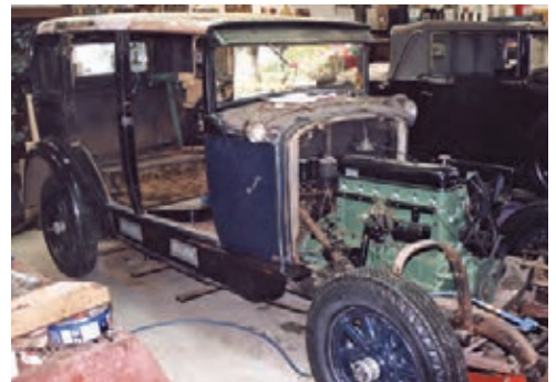
Motor done, wood finished, "new" valances.
