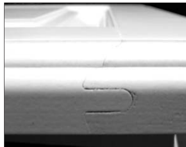
Example of end joint separation
