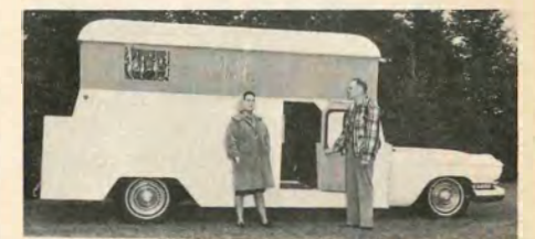
"Mac" McGladrey of Cloquet, Minnesota grafted a typical chassis type camper onto a 1959 Cadillac . . . and then raised the roof!
