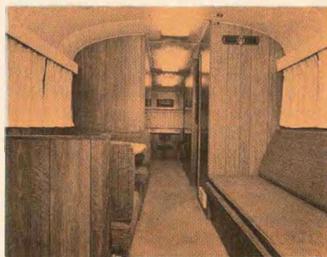
ONE OF THE UNIVERSAL FEATURES of motorhomes is a floorplan with a center aisle and a bathroom on the side. Above is front to rear view of a Coachette unit.
