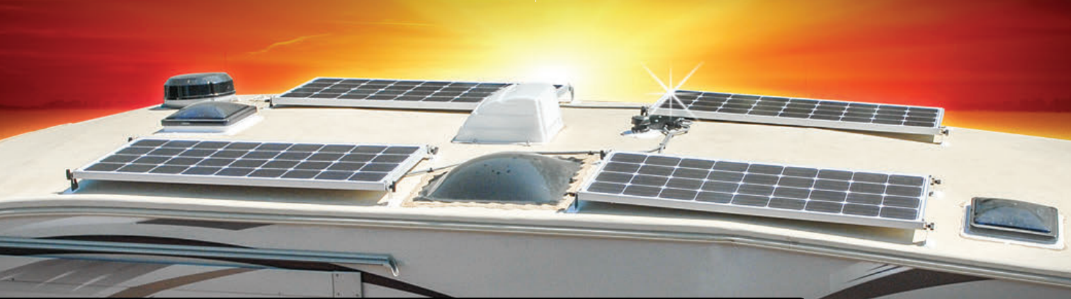
The four 160-watt solar panels fit nicely on the front section of the fifth-wheel, and wiring is mostly concealed.
