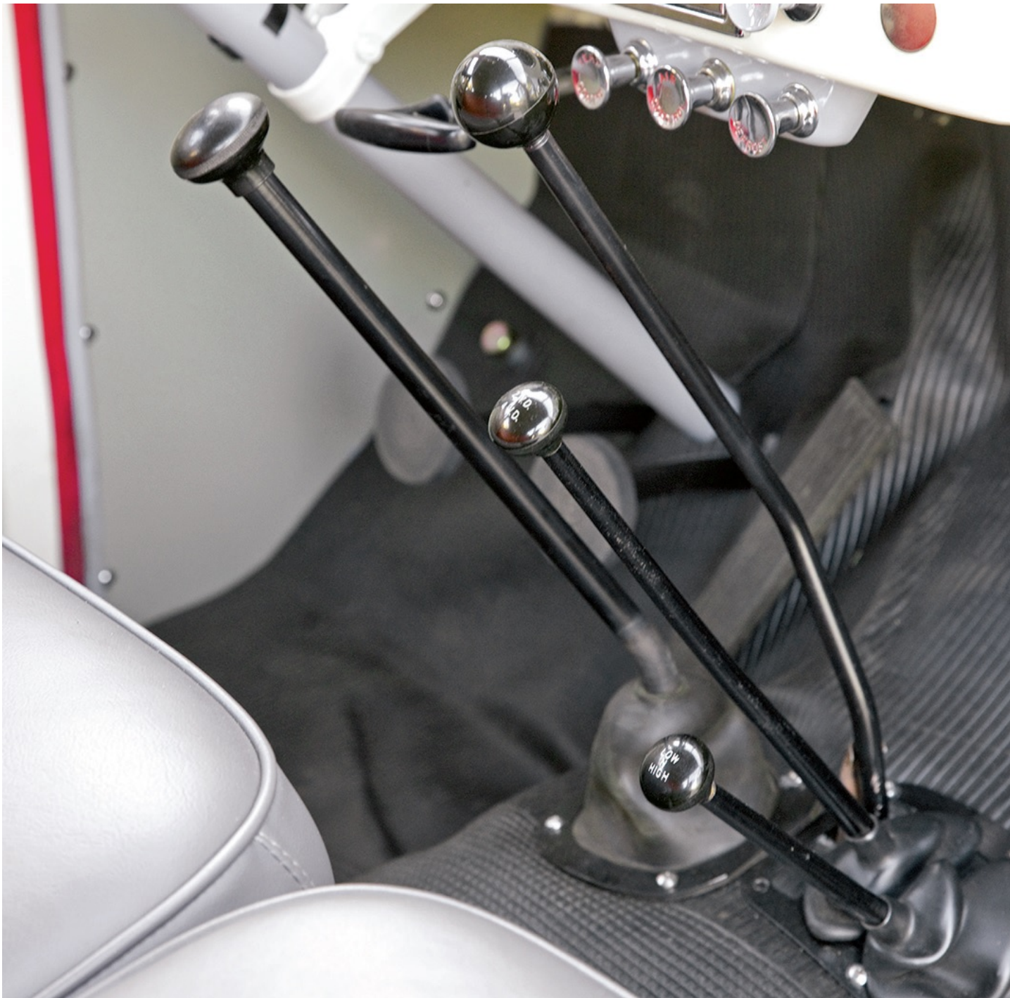
Four shifters control the three-speed transmission, overdrive, 2WD-4WD, and transfer case.
