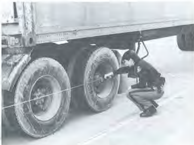
Measuring axle spacing to compute allowable weight.
