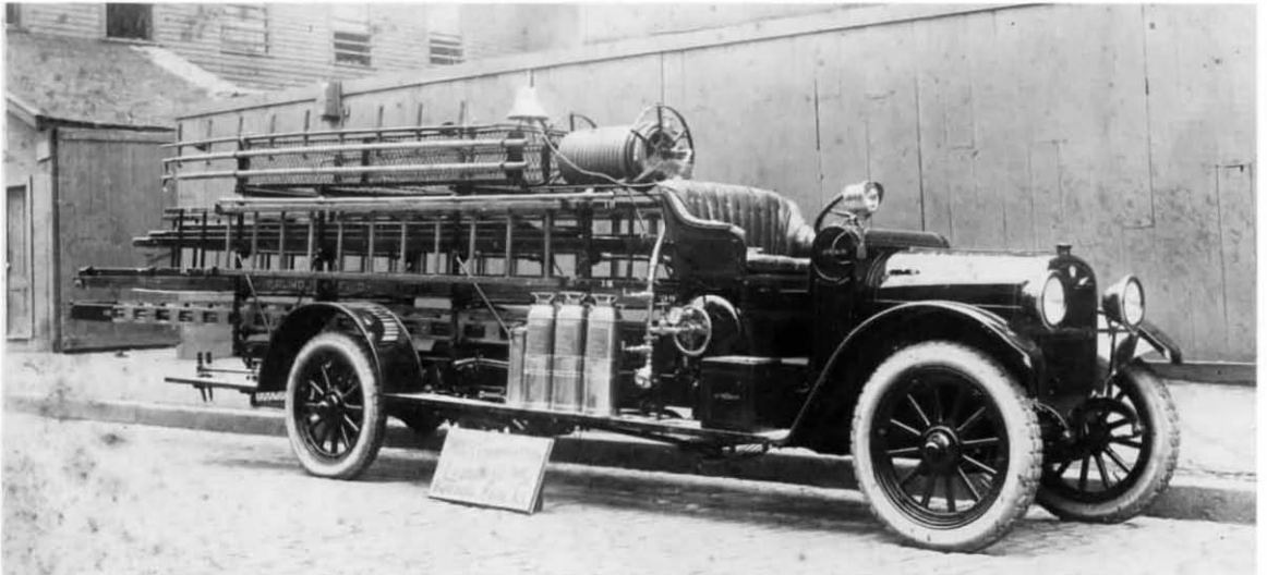
First Falmouth Ladder 2 Chemical, on Reo chassis, vintage 1922. Courtesy Falmouth Fire Department.
