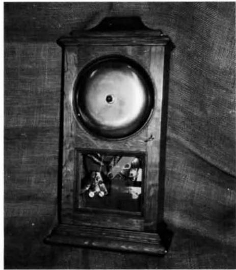
Typical Tapper of early period, made by Gamewell Co., brought alarm signals into officers' homes. Restored by John D. Todd. Courtesy John D. Todd.
