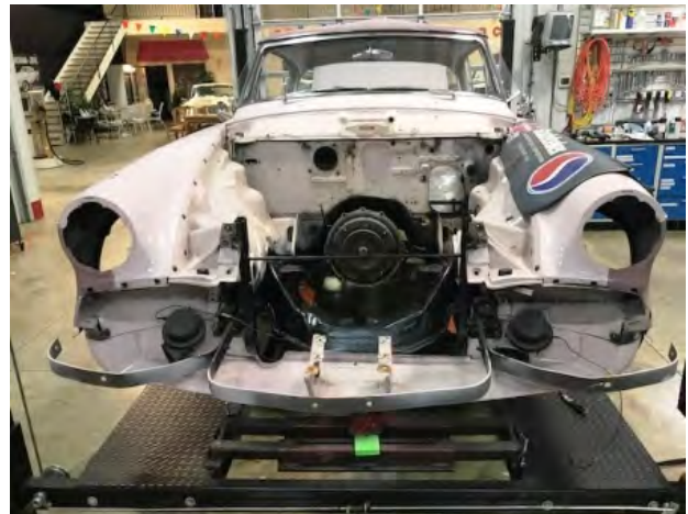
Firewall on a Los Angeles built car matches the inner fender aprons (Accent Color)
