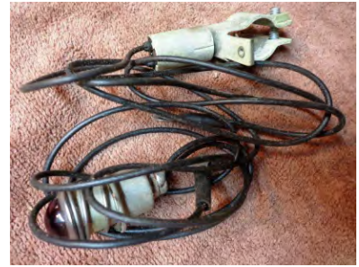
AC-2776 Parking Brake Warning Light
