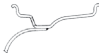
5° DROP CENTER DUAL STEEL WHEEL
