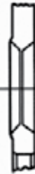
Chamfer extruded on side opposite nut. Causes: Too much torque or improper nut.
