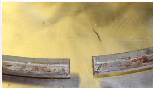
Gap between locking ring ends - Locking ring to be scrapped
