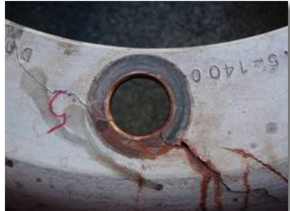
Wheel disc cracks at stud hole
