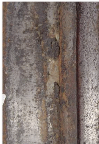
Rim flange wear due to overloading
