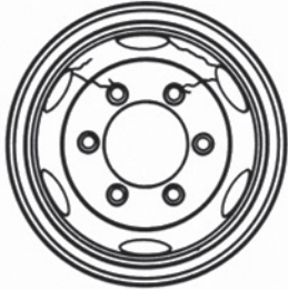
Handhole to handhole. Handhole to bolt hole. Handhole to rim. Cause: Overloading.
