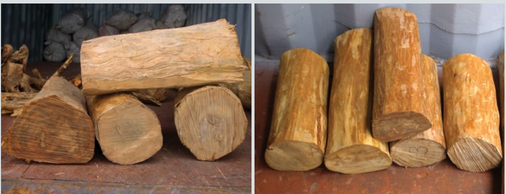
Figure 10.14 Carving logs de-sapped (left), totally clean heartwood logs, near circular in cross-section, with a smooth surface and no hollows, cracks or knots (right)
