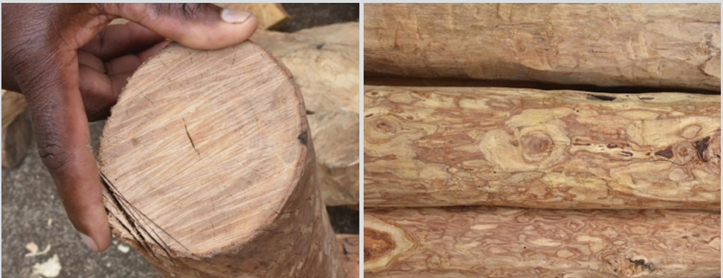
Figure 10.13 Waterwood – sandalwood with incomplete, uneven or wounded heartwood development (transition wood) or heartwood that has been damaged
