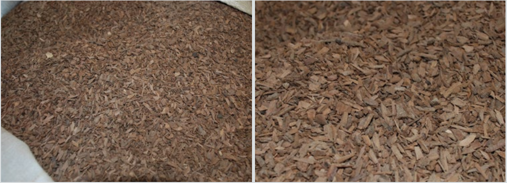
Figure 10.16 Heartwood is milled to a consistent size specification (grade) of 3–5 mm, which is then used for extraction of oil
