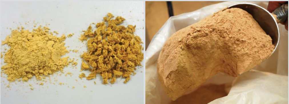
Figure 10.17 Heartwood is milled into a fine powder so that it can be used in the manufacture of joss sticks and other incense products
