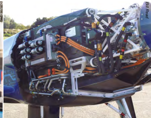
Above left: The Spirit of Innovation is powered by over 6,000 battery cells. Above right: The batteries of the Spirit of Innovation (left) power the three electric motors.
